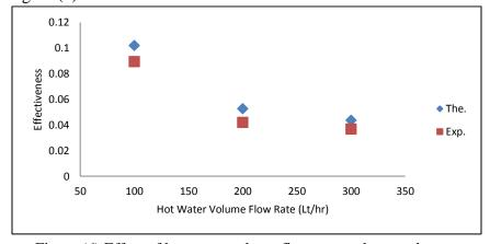
Figure (6) Effect of hot water volume flow rate on heat exchanger effectiveness.
