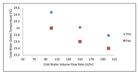
Figure (7) Effect of cold water volume flow rate on cold water outlet temperature.
