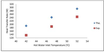
Figure (12) The relationship between heat transfer rate and hot water inlet temperature.
