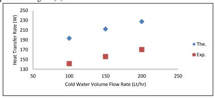
Figure (9) The relationship between heat transfer rate and cold water volume flow rate.
