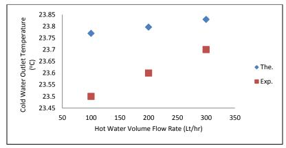
Figure (3) Effect of hot water volume flow rate on cold water outlet temperature.
