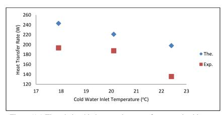
Figure (16) The relationship between heat transfer rate and cold water inlet temperature.
