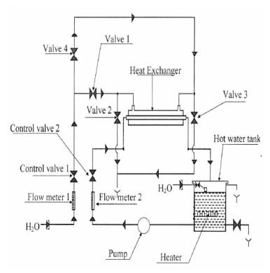
Figure (1) General layout of The Experimental Test Rig.
