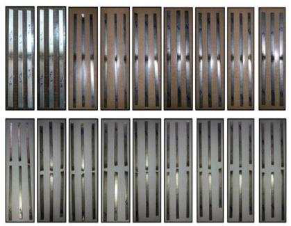
Figure (5). Specimens after tensile test
