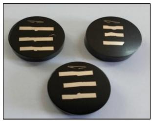
Figure (6). Specimens for micro-hardness test
