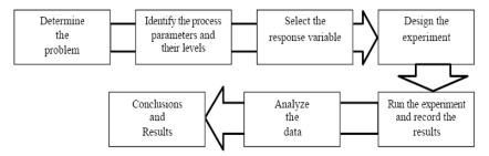
Figure 4. The flow chart of the quality improvement of the process [25].
