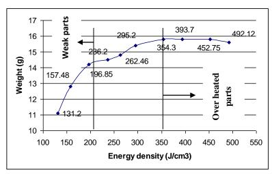
Figure 9. The range of energy density for layer thickness 0.1mm.
