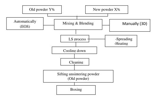
Figure 2. Flow chart of the powder in LS machine [20].
