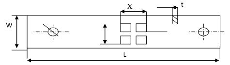
Figure 7. The dimensions of test part specimen.
