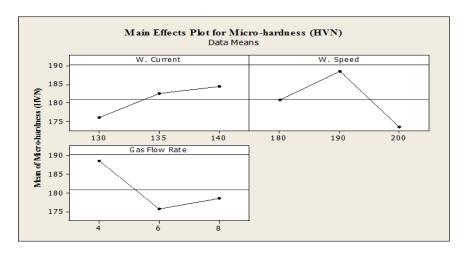
Figure (8). Main effect plots for micro-hardness (HVN)
