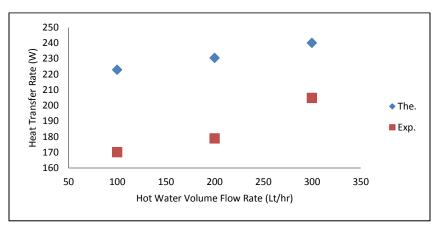
Figure (5) The relationship between heat transfer rate and hot water volume flow rate.
