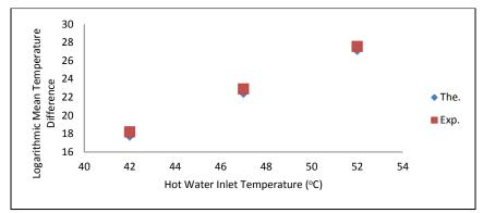
Figure (13) Variation in logarithmic mean temperature difference with hot water inlet temperature.
