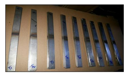
The tensile test was carried out on Zwick universal tester machine with 1000KN load capacity. Nine specimens were tested at each condition, three samples for each specimen as shown in Figure (5). The results of average ultimate tensile strength are given in Table (5).
