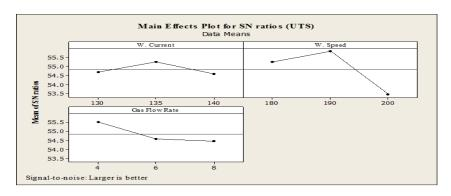
Figure (9). Main effect plots for S/N ratio of ultimate tensile strength (MPa)
