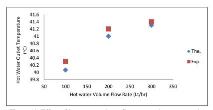
Figure (4) Effect of hot water volume flow rate on hot water outlet temperature.
