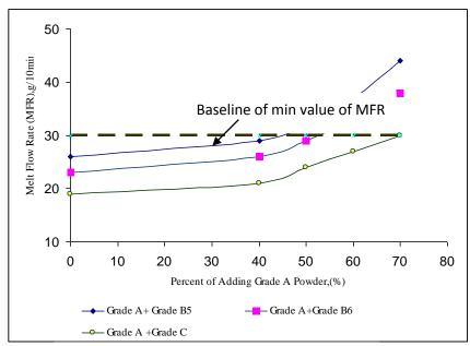
Figure 15. The MFR of B5 to B6 powder grades mixed with different Ratio of virgin powder.
