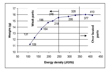
Figure 10. The range of energy density for layer thickness 0.12mm.
