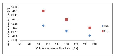
Figure (8) Effect of cold water volume flow rate on hot water outlet temperature.
