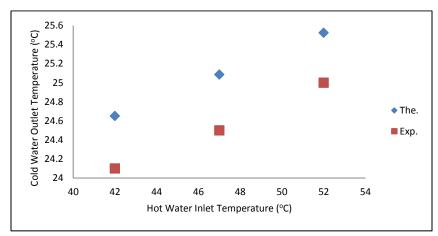
Figure (10) Effect of hot water inlet temperature on cold water outlet temperature.
