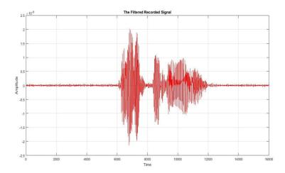
Fig(5): the Recorded Signal (Filtered using FIR filter).
