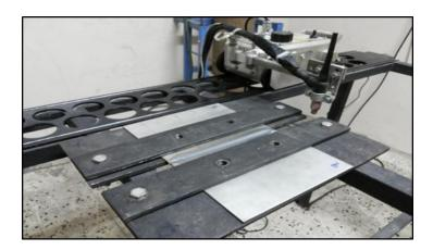
Figure (1). Experimental set-up for TIG welding
