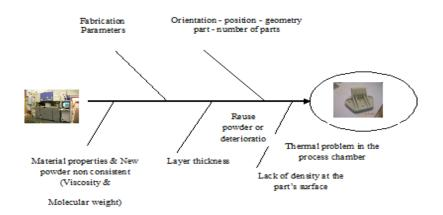
Figure 6. Fishbone diagram of factors influencing the orange peel.
