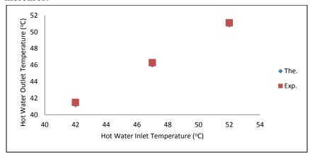
Figure (11) Effect of hot water inlet temperature on hot water outlet temperature.
