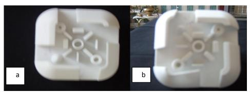
Figure 14. Part fabricated using: a) 21MFR and b) 15MFR powders.
