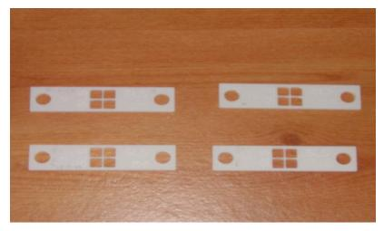
Figure 8. Test parts specimen of the rectangular geometry.
