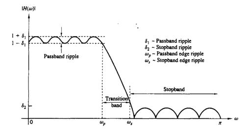
Fig (2): magnitude characteristic of physically realizable filters.
