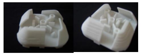
Figure 13. Orange peel texture for the part fabricated using 26 MFR powder.
