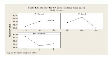
Figure (10). Main effect plots for S/N ratio of micro-hardness (VHN)
