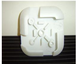
Figure 17. Orange peel texture for the part fabricated using optimum parameters.
