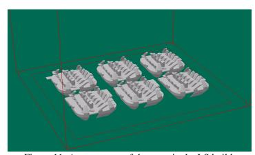
Figure 11. Arrangement of the parts in the LS build.
