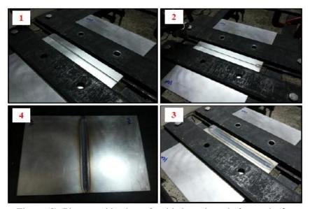
Figure (2). Photographic view of welded specimen before and after welding
