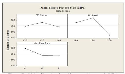
Figure (7). Main effect plots for ultimate tensile strength (MPa)
